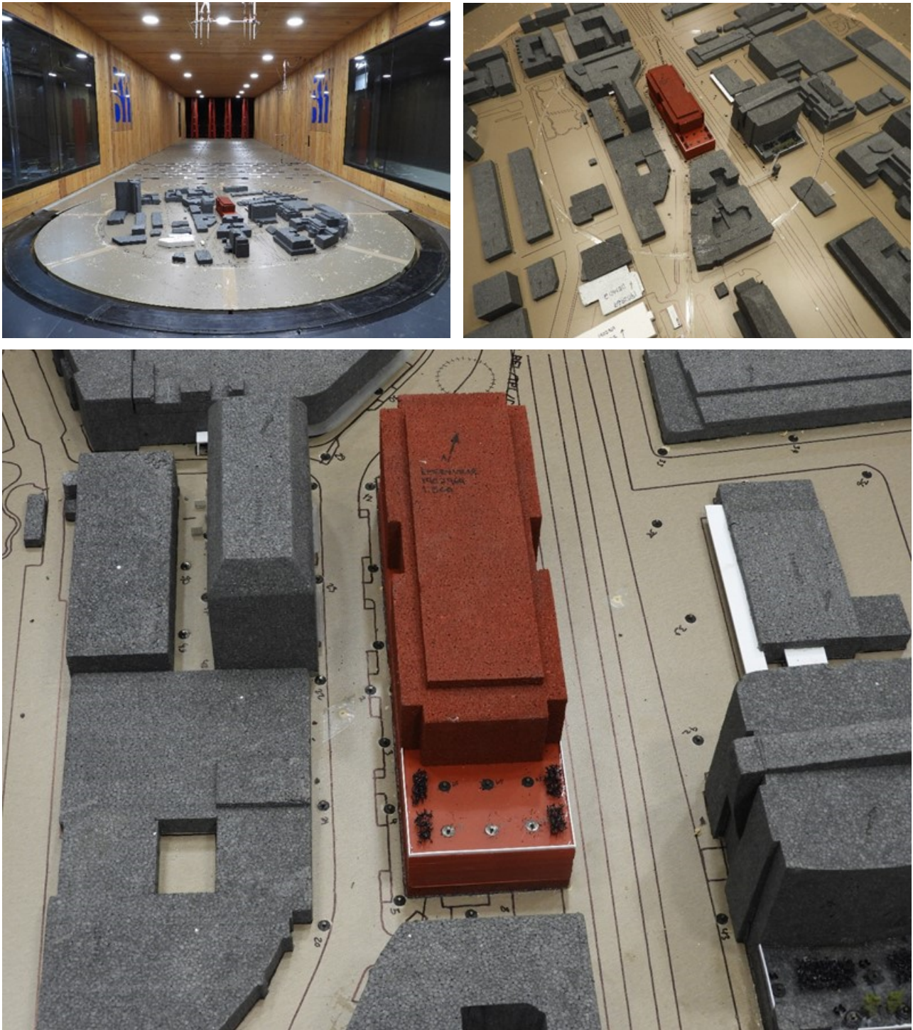
Image 2C: Wind Tunnel Study Model – Alternate G (2020 FDP) Configuration
