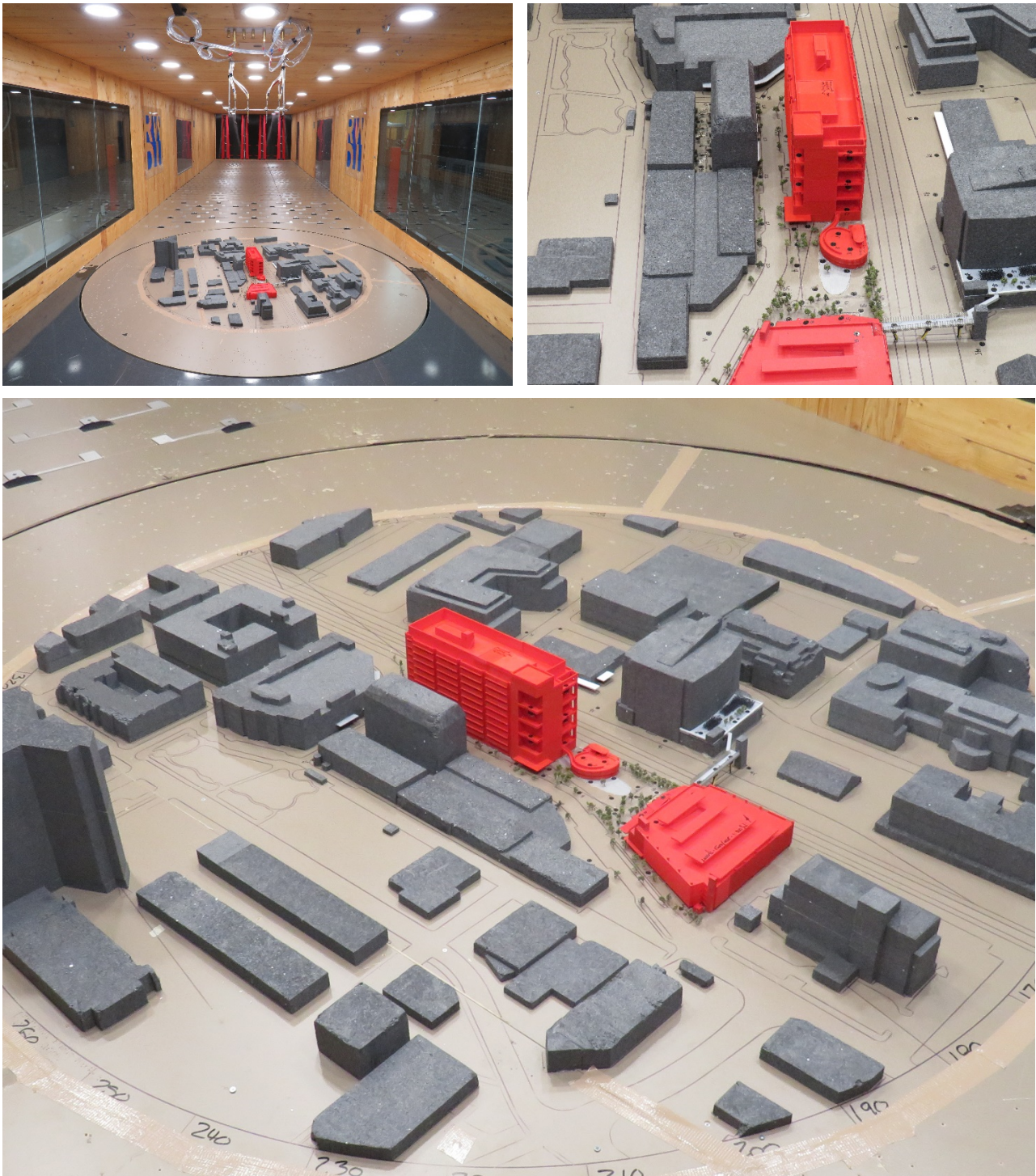
Image 2B: Wind Tunnel Study Model – Proposed Configuration
