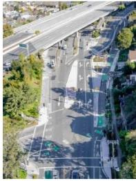
from pedestrians, while still providing clean conforms back to the standard bike lanes. The City pedestrian and bicycle coordinator became "excited about implementing this design." Fehr and Peers assisted Diablo in providing an intersection treatment that provides options to cyclists and proper transitioning along with signal operations and timing to serve the various vehicular, bicycle and pedestrian users.
