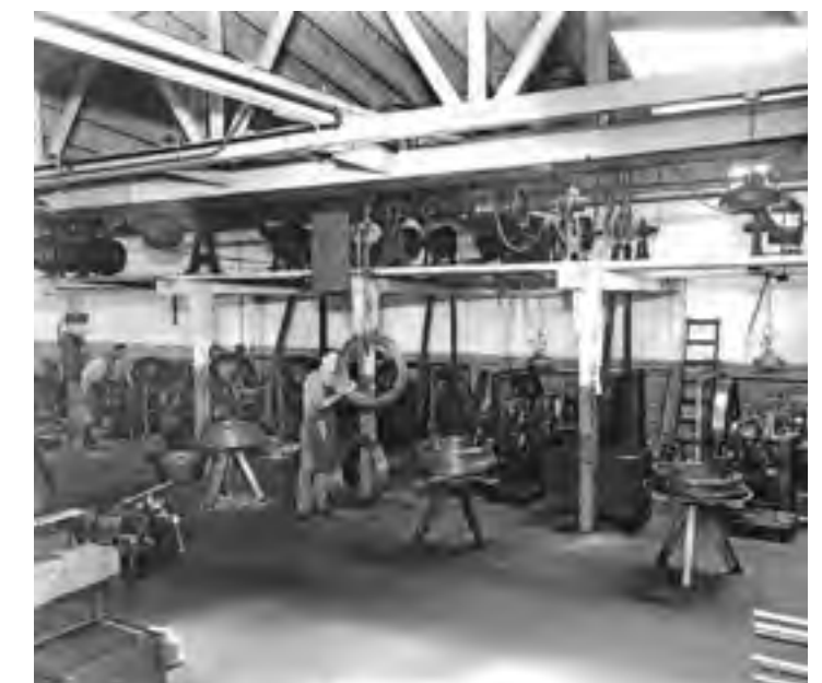
Albert Wright Co. overhead pulleys transfer power to machinery on floor | image source: (EHS) Photo Archive
